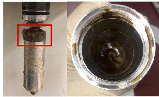
Fig. 4. A gelled portion of samples placed on top of the rheometer bob after  $193.4^\circ\text{C}$  test (left), and a portion of mud sample with a high concentration of burn Cedar Fiber in the bottom of the sample cup (right).
